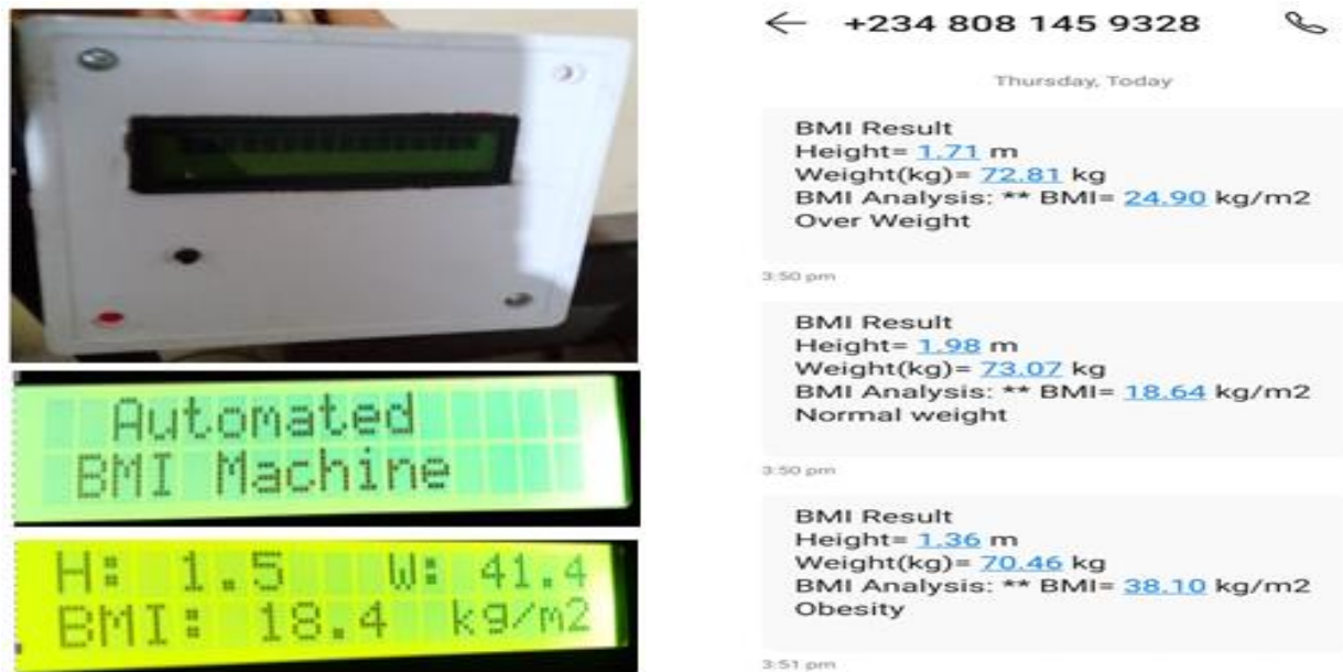
Figure 5: (a) LCD Interface at Different States (b) Backend Confidential Communication between GSM module and Microcontroller
