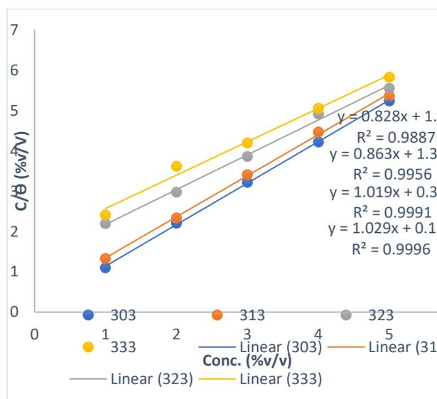
Figure 4. Langmuir adsorption isotherm plots for LTLE on mild steel in 0.5 mol/dm<sup>3</sup> HCl.
