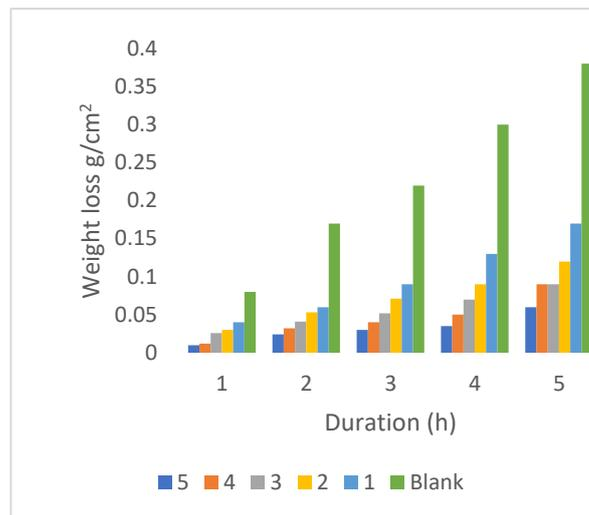
Figure 1. Impact of contact duration on weight loss of mild steel in 0.5 mol/dm<sup>3</sup> HCl at 303 K
