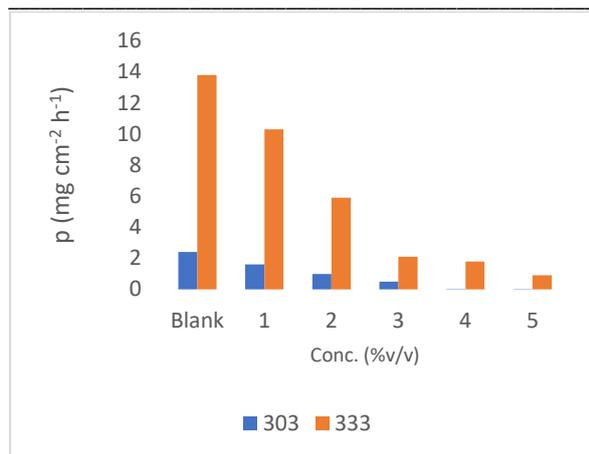
Figure 3. The change in corrosion rate with different concentrations of the inhibiting agent for mild steel in 0.5 mol/dm<sup>3</sup> HCl with *L. taraxacifolia* at temperatures of 303 K and 333 K.
