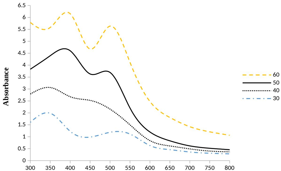
Figure 5: The UV-Visible spectrum of synthesised TC-AgNPs at different temperature intervals
