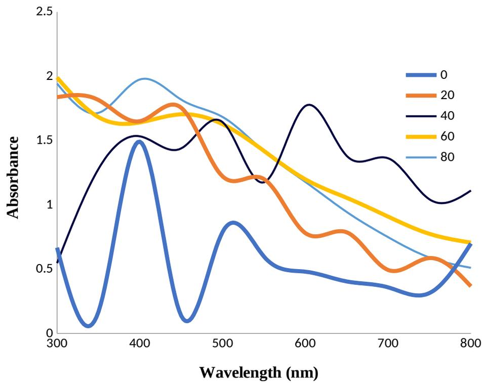
Figure 4: The UV-Visible spectrum of synthesised TC-AgNPs at different time intervals
